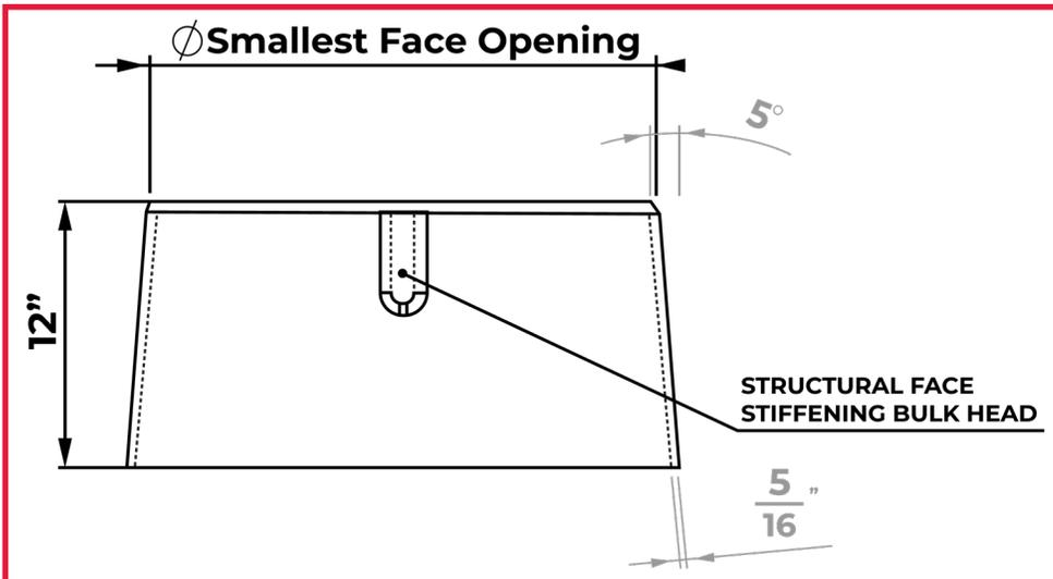
Offered specifically to form an opening in Top Slabs with a lesser wall taper than our Standard Hole Forms for box walls. Their 5° wall taper will net only 2 1/8" diameter growth from face to largest opening on 12" slab thickness.
